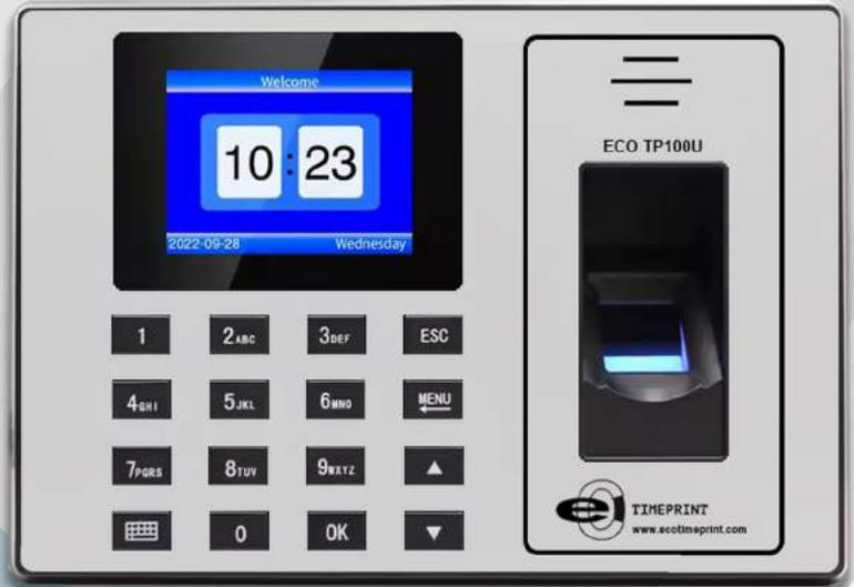
ECO TP100U is a basic and easy-to-use time attendance device with a built-in attendance report feature. It supports fingerprint and passwort verification, with a capacity for 1,000 users and 100,000 records. This device is suitable for small businesses, offering reliable and efficient attendance tracking. Its compact design and user-friendly interface make it a perfect fit for organizations looking for a cost-effective solution to manage employee attendance.
