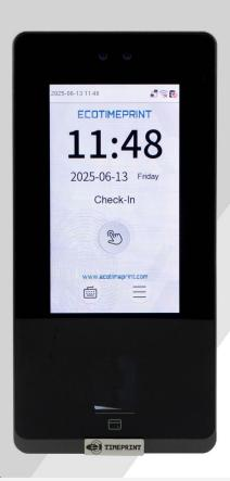
ECO SF300 Pro is a time attendance and door access terminal that supports multiple authentication methods, including face recognition, fingerprint, PIN and ID card. What makes it unique is its slim, modern design, which seamlessly fits into any professional environment. With Visible Light Technology, it can detects human faces from greater distances and higher speeds, ensuring quick and accurate recognition.
