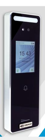
ECO SF200 is a time attendance and door access terminal that support both face and fingerprint authentication. Its distinctive compact design sets it apart in our Smartface series. Utilizing Visible Light Technology, this terminal automatically performs recognition for a target from an extended distance, activating upon detecting a human face within its range. This results in superior recognition quality, enhancing both speed and accuracy
