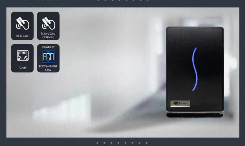
ECO200D is an IP based RFID access control devices, which is made with elegant design and professional surface treatment. The device has lock control, alarm, exit button, door sensor. The Wiegand-in interface is used to connect external reader to construct master and slave system. The operation can be done on PC software and upload to the device through TCP/IP, RS232/485 communication.
